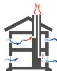
Figur 2. S-system (Svensk Ventilation, 2017a)
